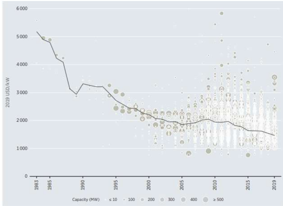
Figure 5-4: Total installed costs of onshore wind projects and global weighted average, 1983-2019 (Ref. 13)
