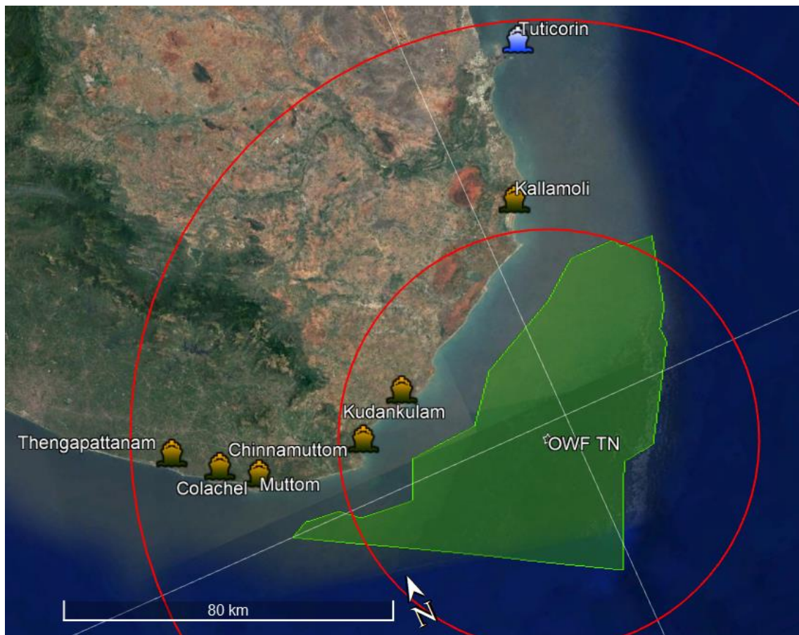
Figure 66: O&M Ports – Potential O&M bases for Tamil Nadu OWZ. Red curves denote 50km and 100km radius from OWZ central point.
