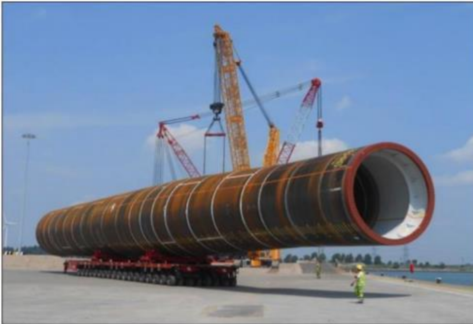
Figure 78: Transportation of monopiles with SPMT
