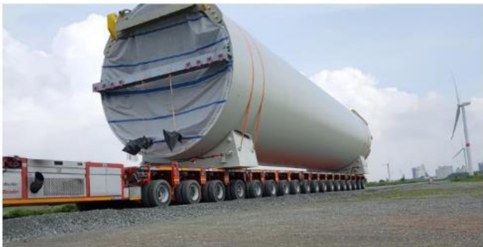
Figure 79: SPMT for transportation of large and heavy components
