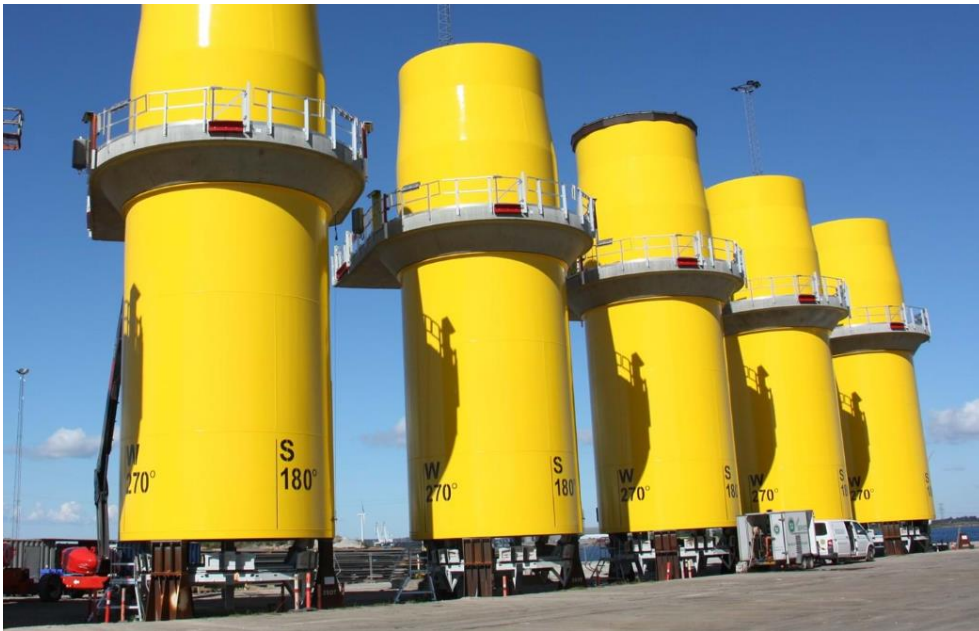
Figure 84: Storage of transition pieces. Bladt Industries
