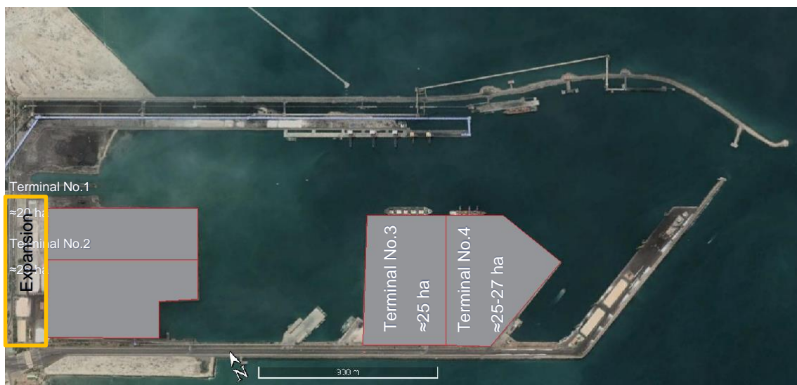
Figure 24: Tuticorin Port – OW Terminal Vision Inner harbour transformed to OW hub (doubling for project cargo, break bulk, etc) with outer harbour focused on container traffic – Tuticorin port.
