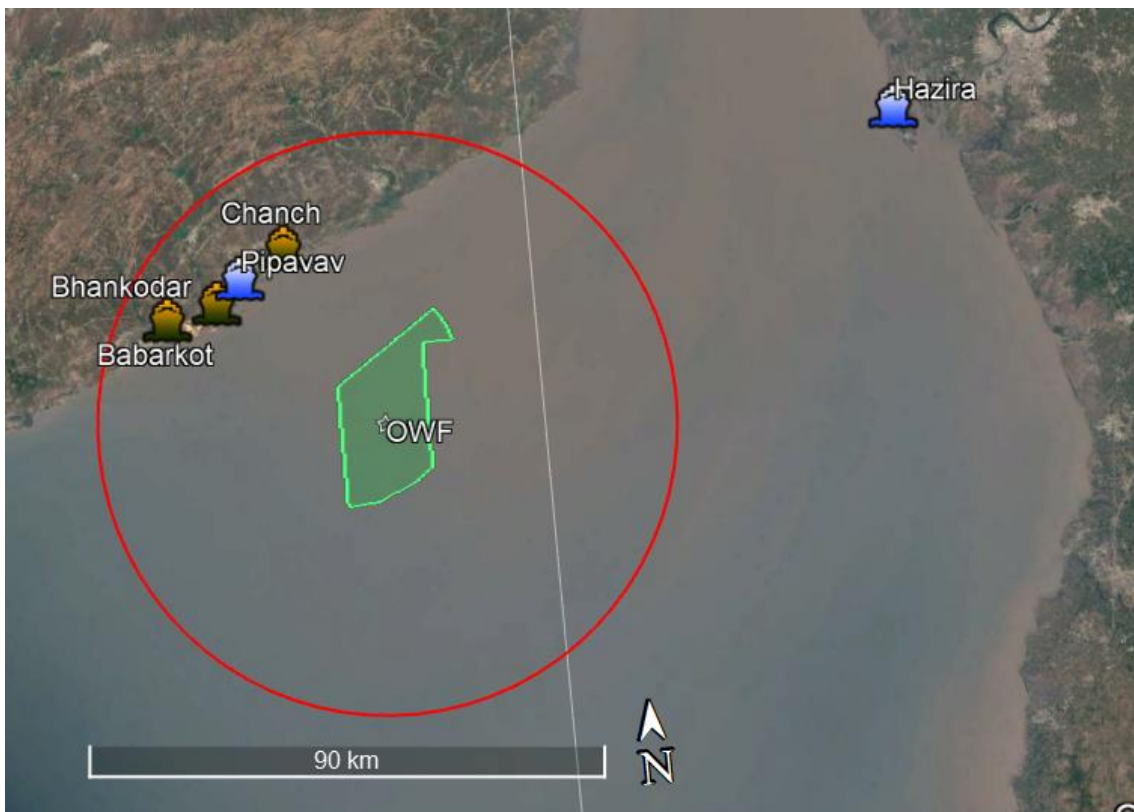
Figure 67: O&M Ports – Potential O&M bases for Gujarat OWZ. Red curve denotes 50km radius from OWZ central point.
