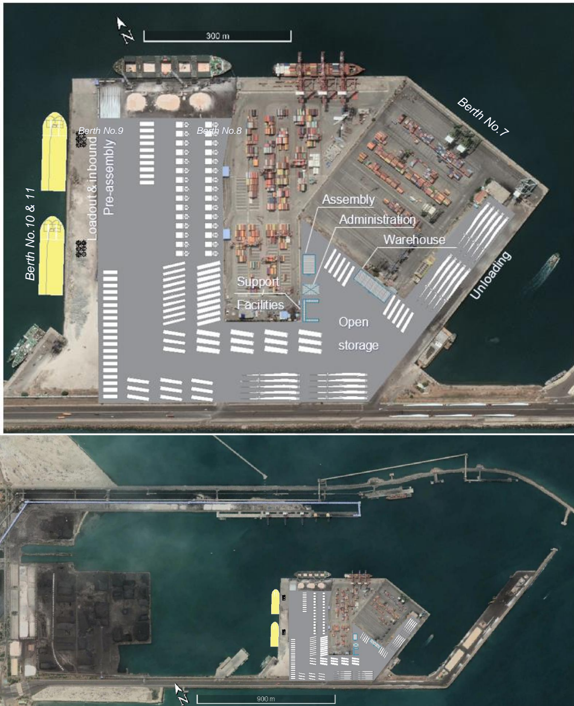
Figure 21: Tuticorin Port – OW Terminal Alternative 1 Future general cargo terminal suitable for OW installation adjacent to Berths 5-9
