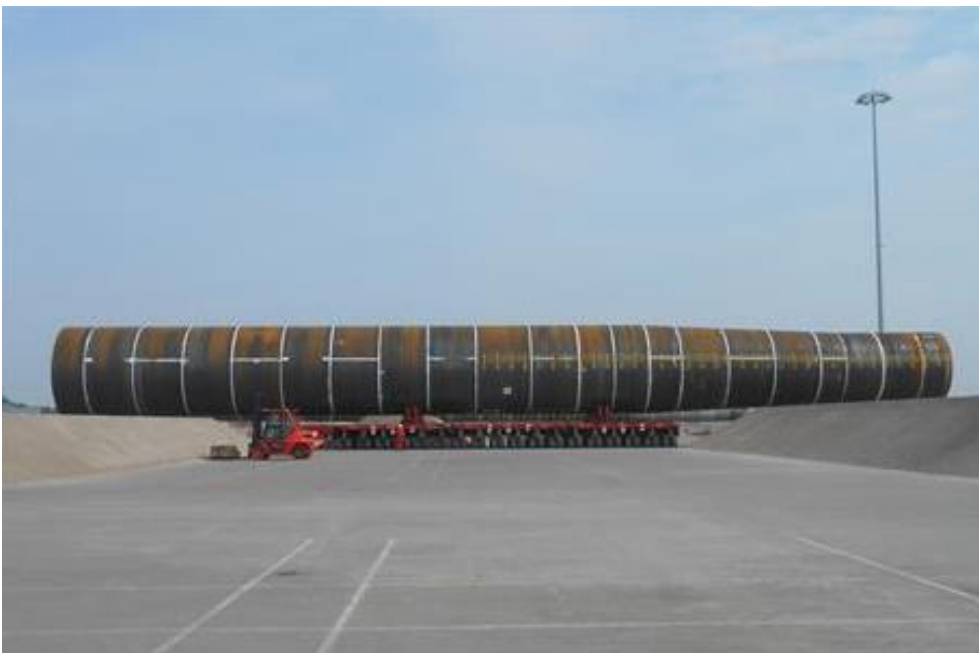
Figure 83: Monopile stored on earth embankments
