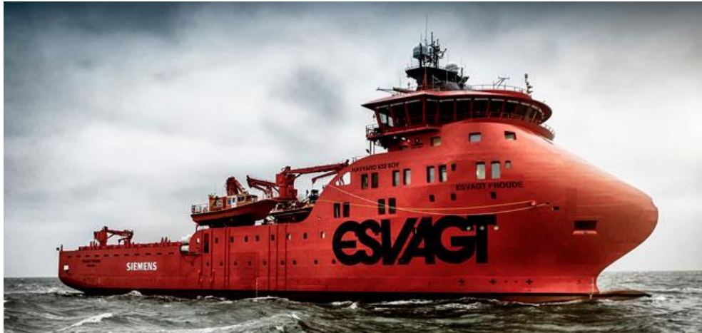
Figure 5-4 | Service Operation Vessel used by Siemens for servicing offshore wind farms (Esvagt, n.d.)
