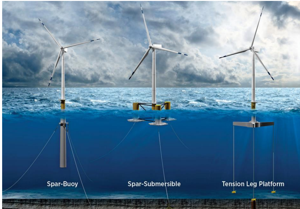
Figure 2-3| Visualization of different types of floating foundations (NREL, u.d.) in the concept/system sub-report)
