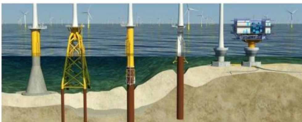
Figure 2-2| Overview of fixed bottom design concepts (COWI, 2021)
