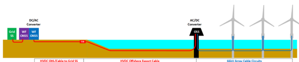
Figure 2.53 - HVDC export cable from offshore substation
