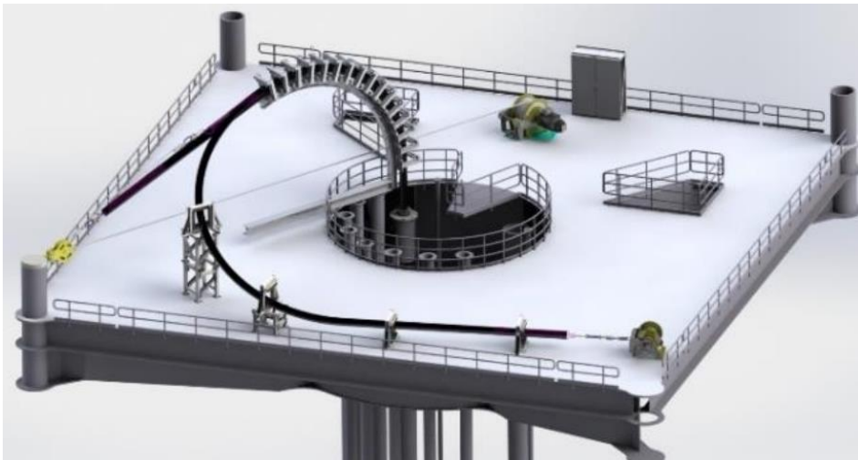
Figure 31 OSS Cable Pull-in Method
